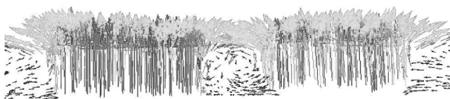
Fig. 4 Velocity vector distribution on the plane cutting through the defrosters shows bound vortices.
